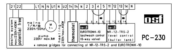
The bridge which is installed by the manufacturer between the terminals 13 and 14 has to be removed if a level control unit INR-12-TRS-2 is connected. If a level control unit is not connected, the bridge has to remain bolted between these terminals. In this case, the terminals 11 and 12 shall not be used.
